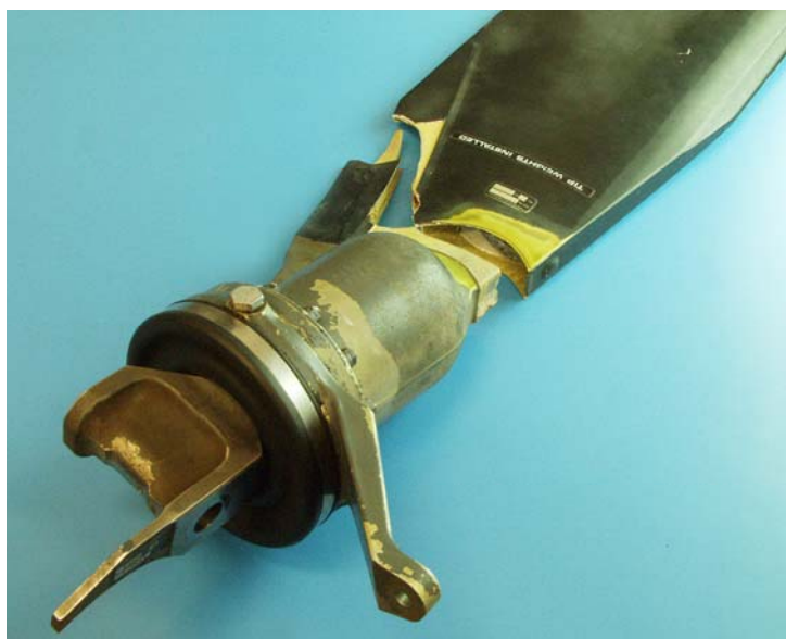
Figure 3: The fractured main rotor blade of VH-OHA
